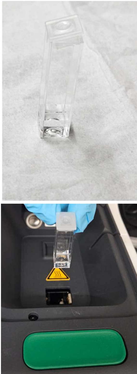
Fig 3. A) Partially capped cuvette. B) Place the sample into the Zetasizer instrument.
