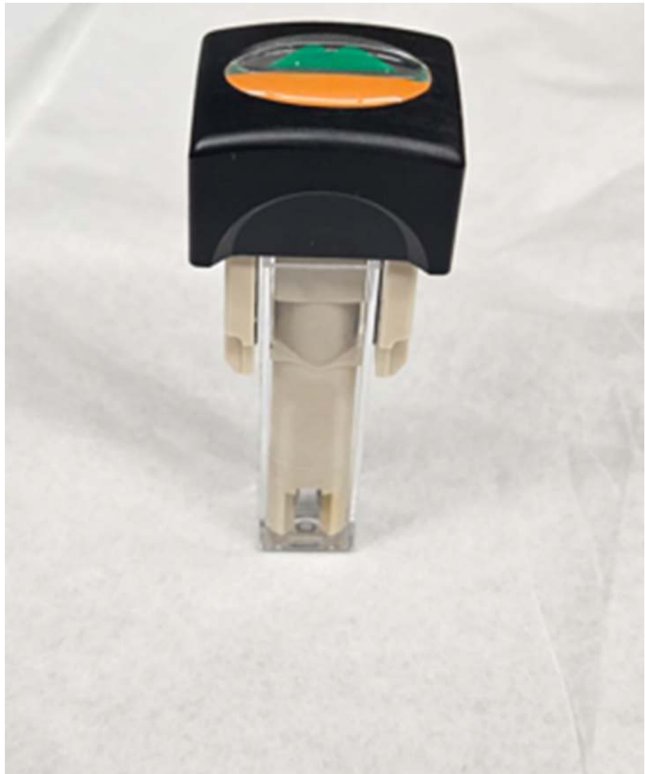
Fig 5. A sample with the dip cell to measure ELS.
