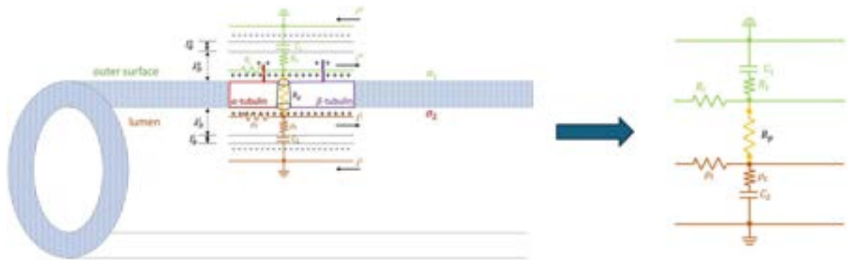
Fig. 10. Multi-scale electrokinetic model for microtubules. It represents the outer and inner EDLs as coupled transmission lines (green and brown) connected through nanopores in the microtubule wall (yellow), modeling tubulin as a hollow cylindrical structure.
